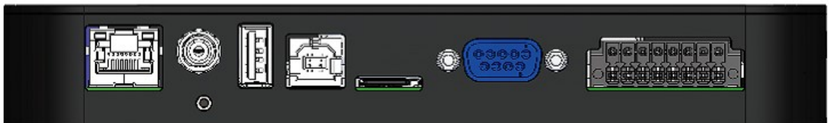
Figure 8 – Power, RS-232, USB, SDCard and LAN Connections
