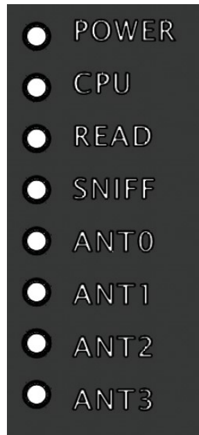
Figure 7 – ALR-F800 Front Panel Reader Diagnostic LEDs
