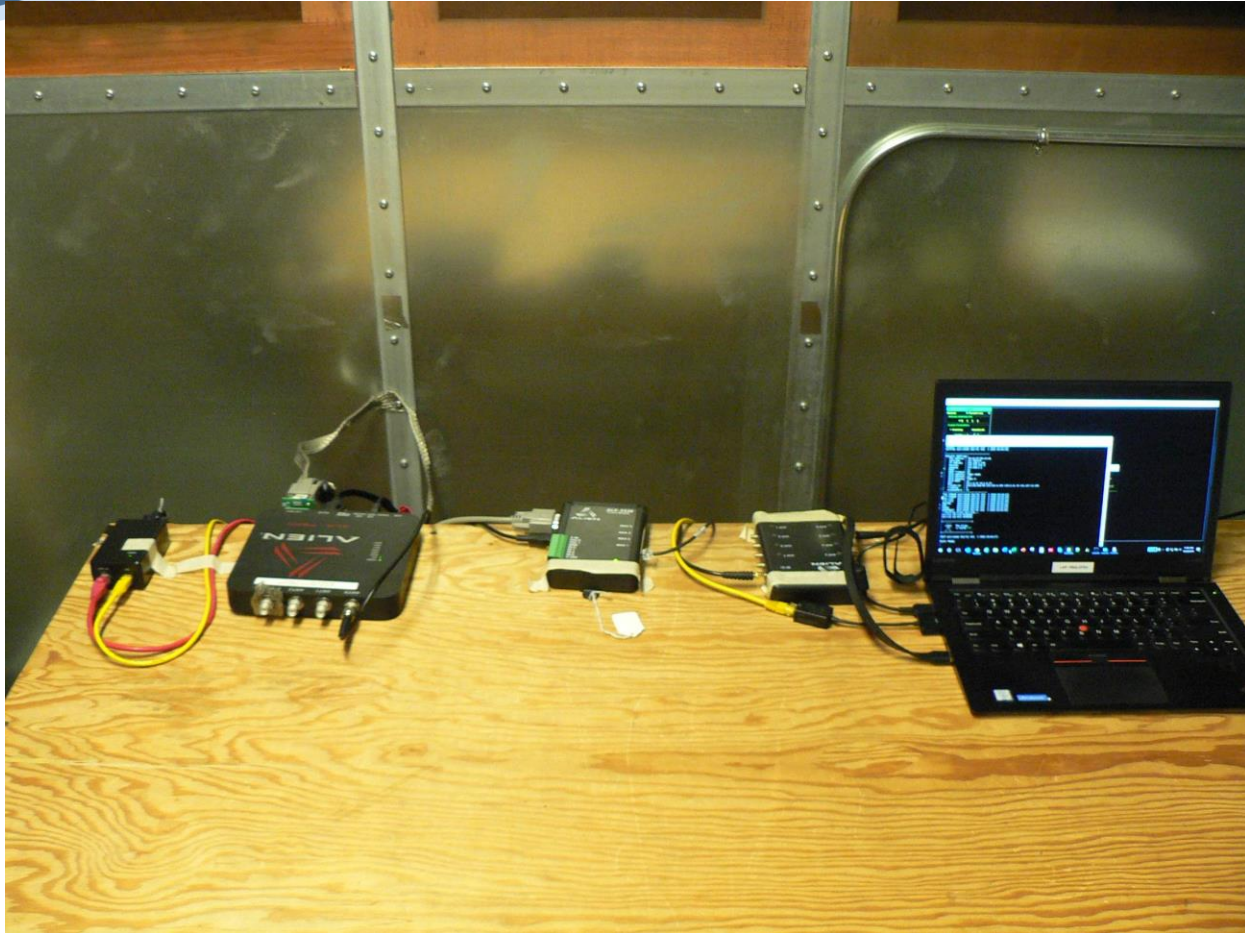
PoE AC Mains Conducted Front
