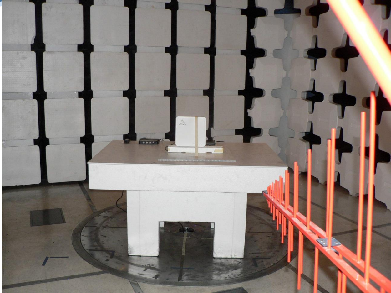
ALR-8698 Antenna TX Spurious 30-1000MHz
