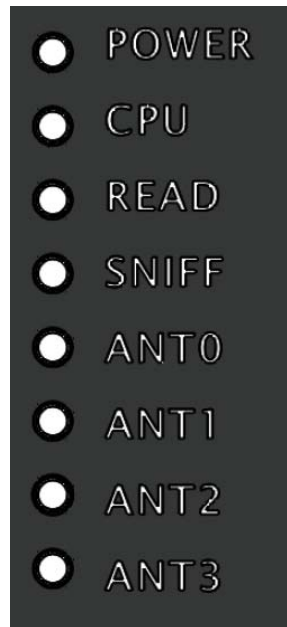
Figure 7 – ALR-F800 Front Panel Reader Diagnostic LEDs
