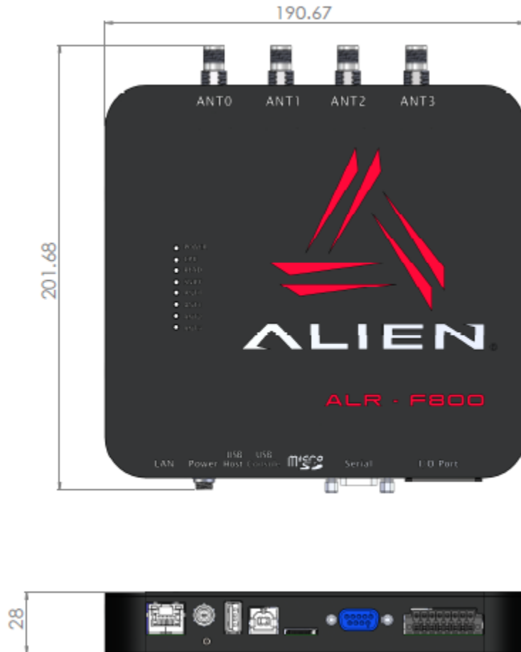
Figure 1 - Outline Drawing of the ALR-F800 (mm)
