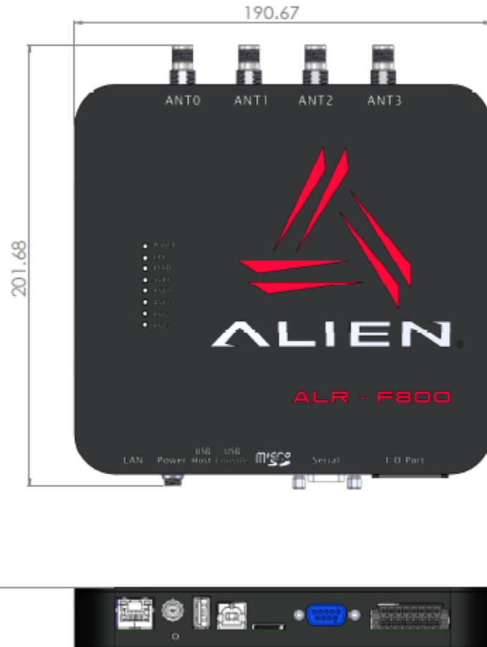
Figure 1 - Outline Drawing of the ALR-F800 (mm)
