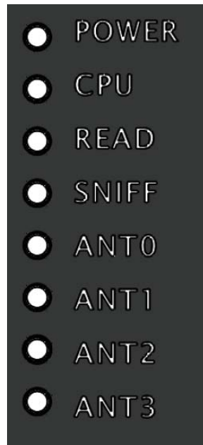
Figure 7 – ALR-F800 Front Panel Reader Diagnostic LEDs
