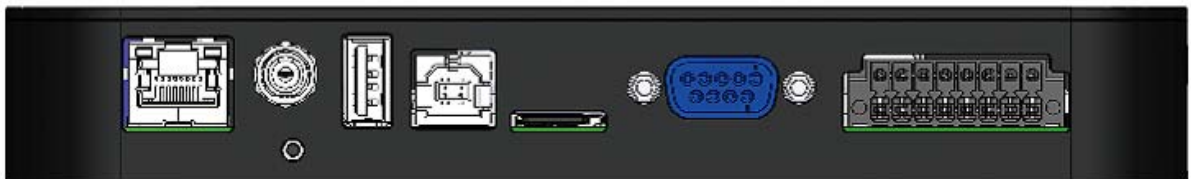
Figure 8 – Power, RS-232, USB, SDCard and LAN Connections
