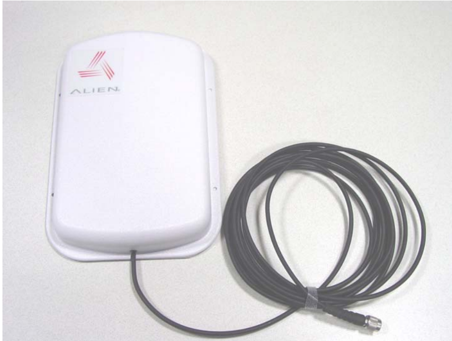
Circular Antenna External View
