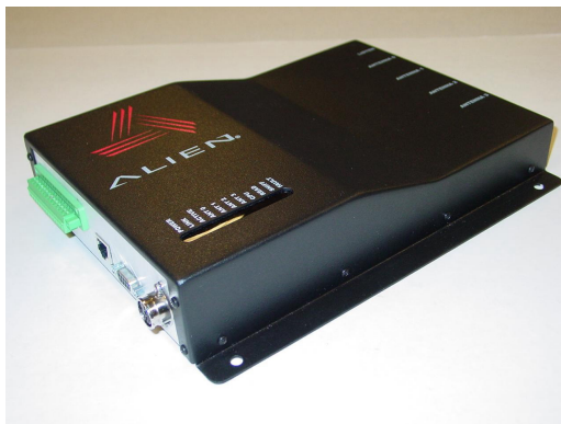
Figure 8 - View of the Reader showing mounting holes
