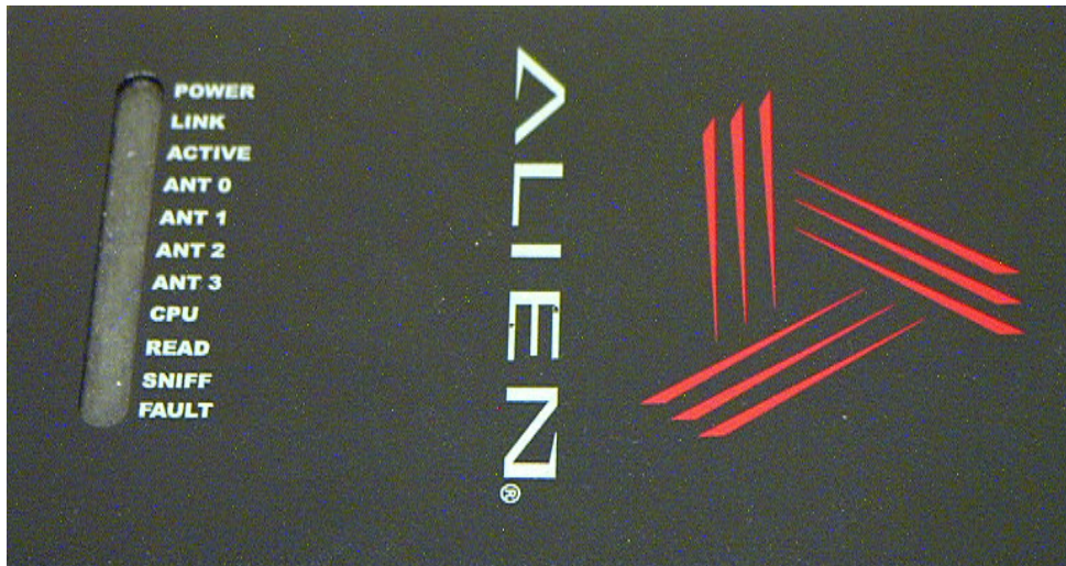
Close up of LED indicators
