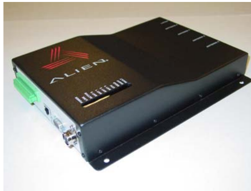
Figure 21 - View of the Reader showing mounting holes
