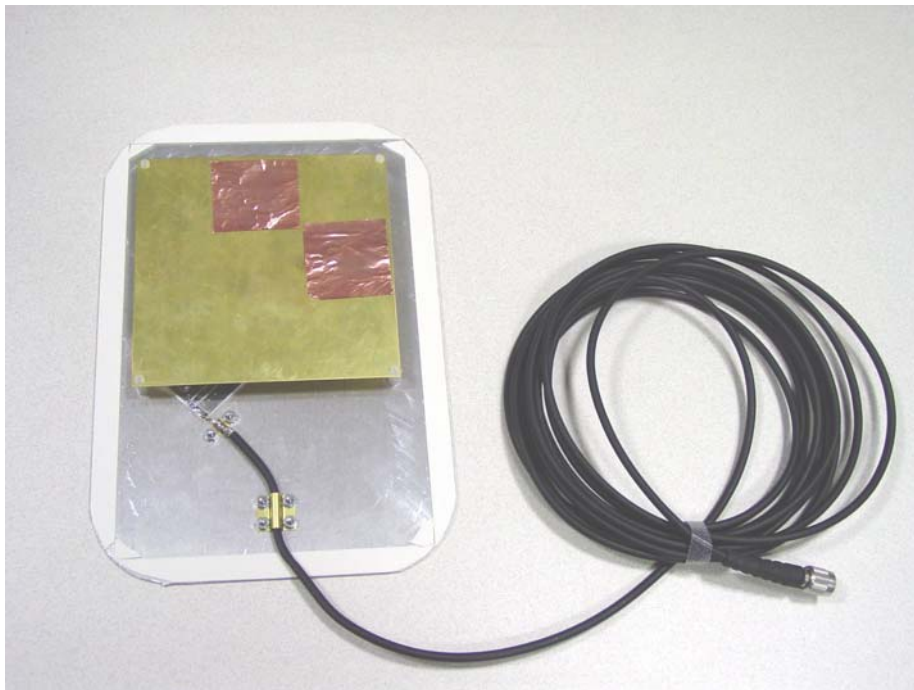
Circular Antenna Internal View
