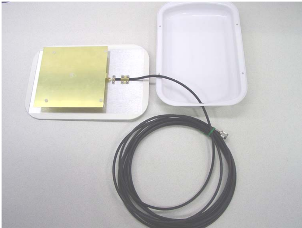
Linear Antenna Internal View
