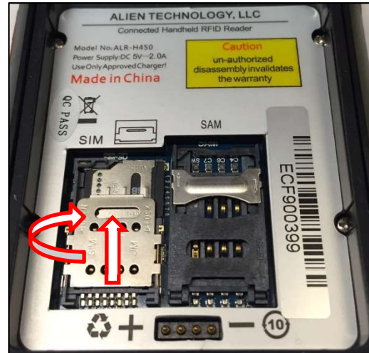
FLIP the SIM card holder back down and SLIDE it upward to lock it in position.
