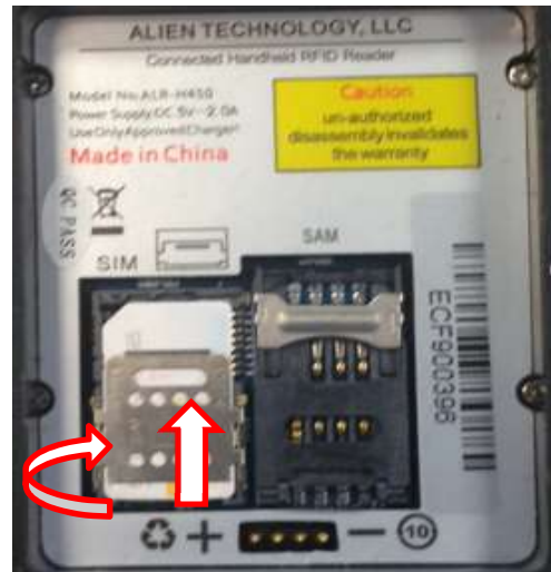
FLIP the SIM card back down and SLIDE the holder upward to lock it in position.
