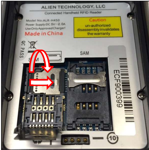
FLIP SD card holder down and slide it toward the right to lock it in position.
