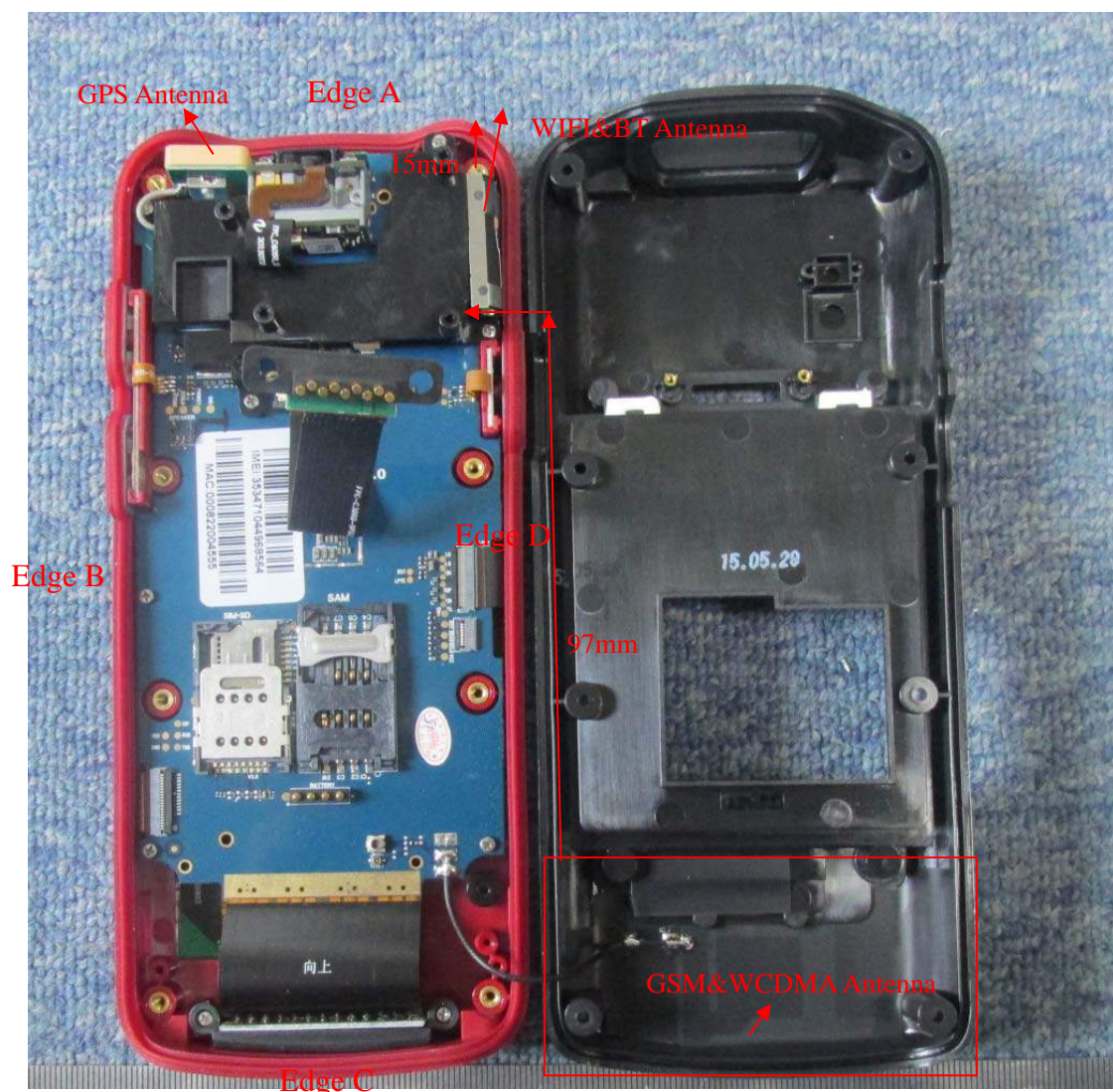
Fig. 3 Position of the antennas
