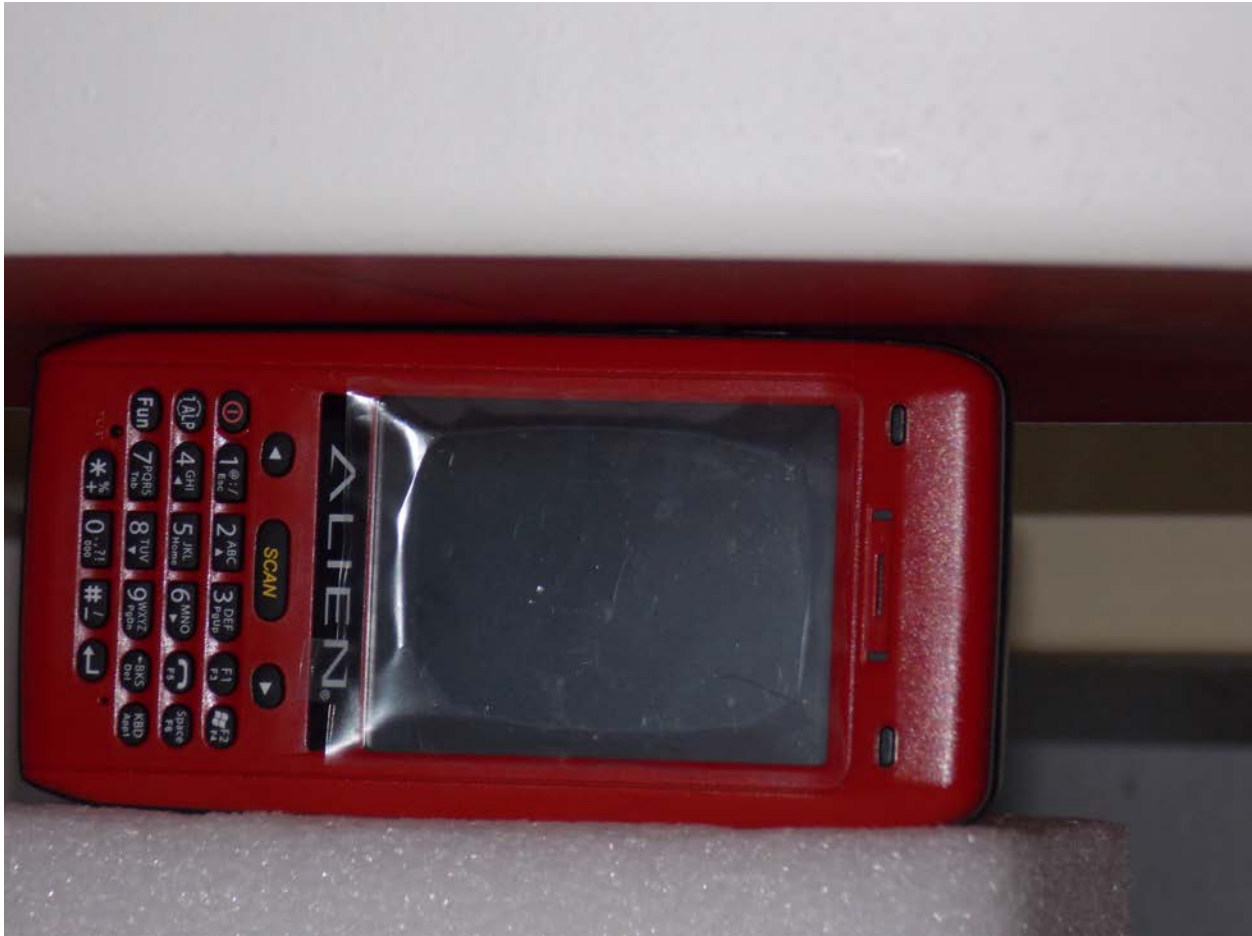
Test Position Side F Without RFID Module 0 mm Gap
