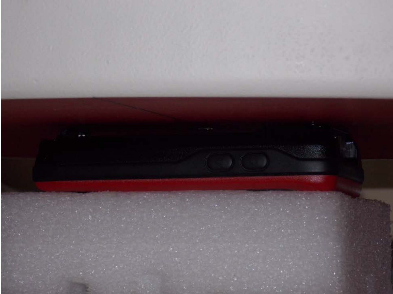
Test Position Side A Without RFID Module 0 mm Gap
