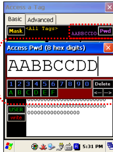
The violet Pwd button opens up a dialog window where you can enter in an Access Password, for accessing tag memory that may have been locked.
