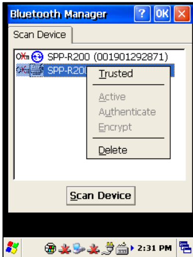
Here we've discovered a Bixolon SPP-R200 mobile printer. Double-tap it and select "Trusted" to set up the link.
