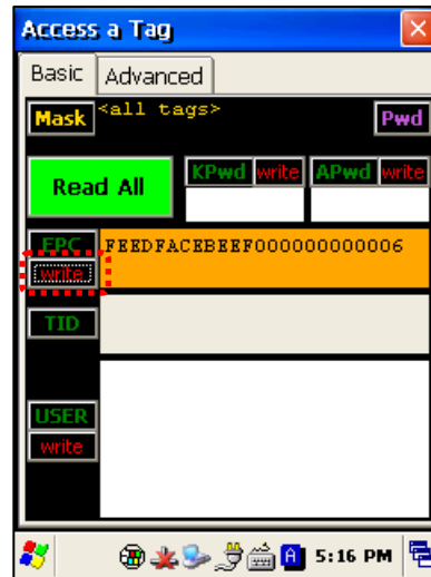
Pressing the red “write” buttons cause the reader to write the shown data to the tag. You can edit the data in the field before writing it to the tag. The field turns orange while writing, and then turns white or red, depending on the success of the write operation.
