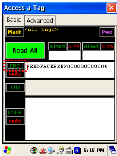
Pressing the small green buttons labeling each memory field will cause the reader to only read data from that field.
