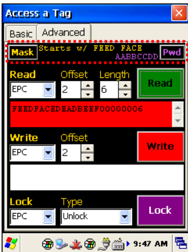
As on the Basic Access tab, you have full access to the tag Mask and current Access Password in this tab. On this screen, the read operation failed for two reasons: the mask doesn’t match the tag’s new EPC (FEEDFACEDEADBEEF...) and we’re trying to access it with an incorrect Access Password.
