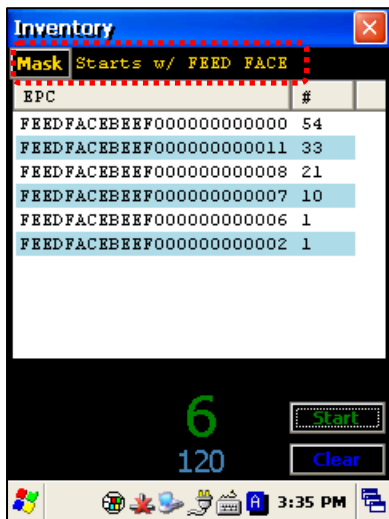
Clicking the yellow Mask button at the top of the Inventory screen takes you to a page where you can specify a subset of tags to read (see the Tag Mask section). This powerful feature causes the reader to only read the tags you want it to read.
