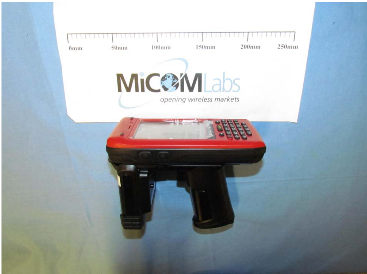
Alien Technology ALH-90XX Handheld RFID Reader
