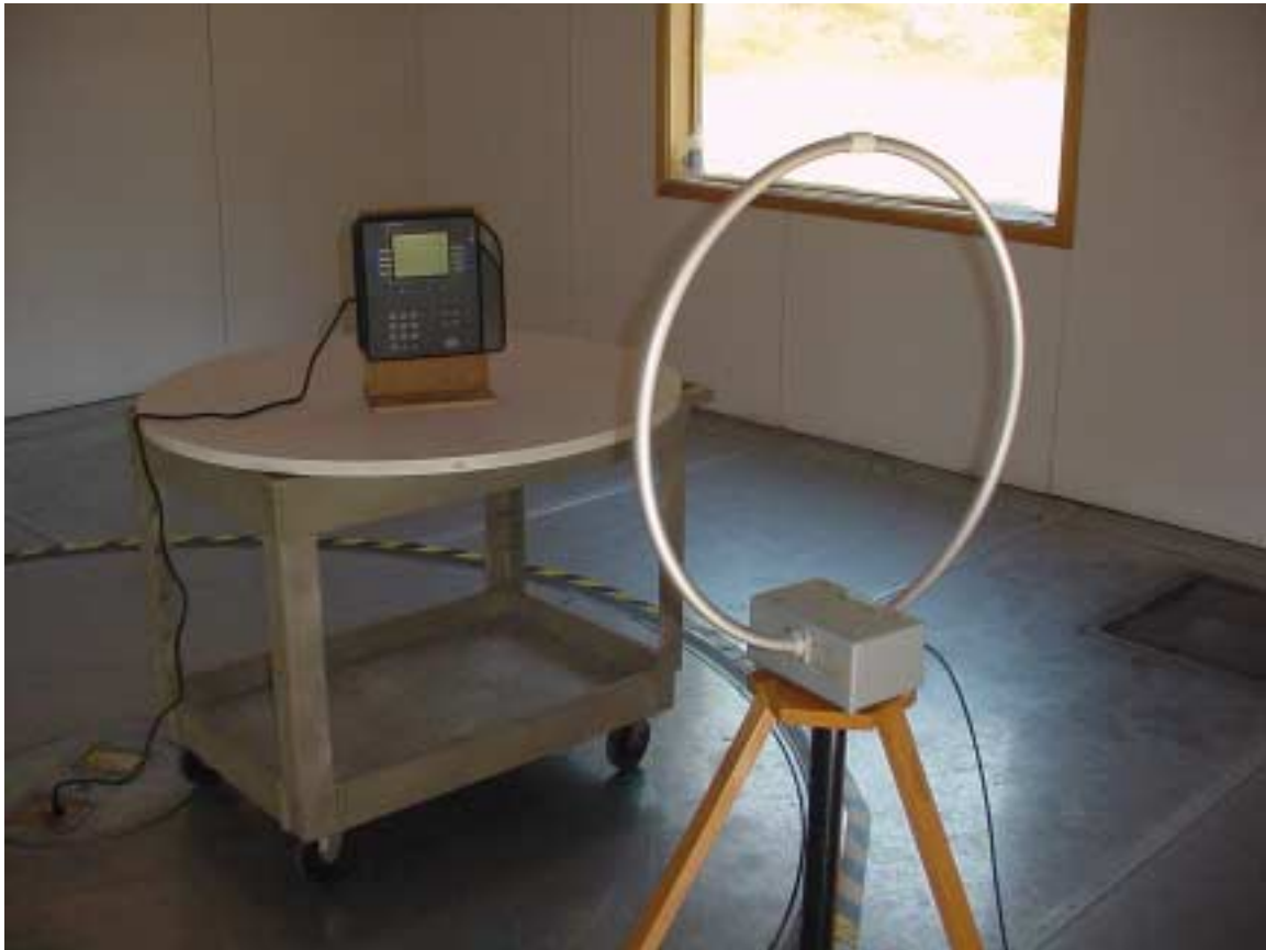
Radiated 1 meter magnetic field setup
