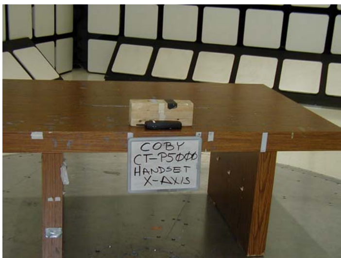
Radiated Emissions – Handset X – Axis 10M Chamber
