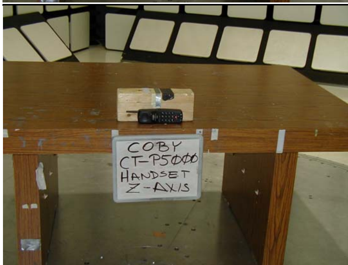
Radiated Emissions – Handset Z – Axis 10M Chamber
