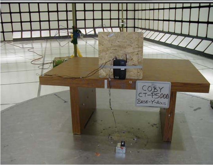
Radiated Emissions – Base Y – Axis 10M Chamber
