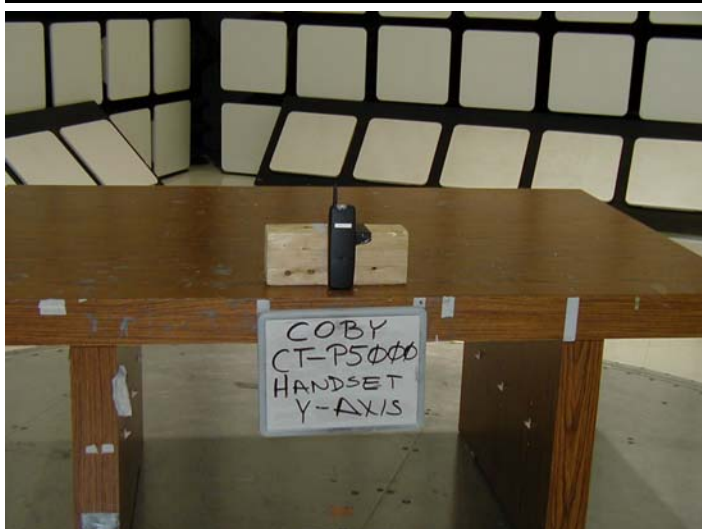
Radiated Emissions – Handset Y – Axis 10M Chamber
