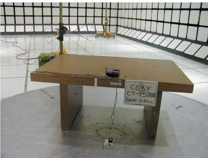
Radiated Emissions – Base X – Axis 10M Chamber
