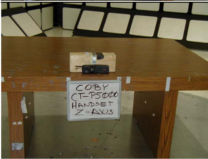
Radiated Emissions – Handset Z – Axis 10M Chamber
