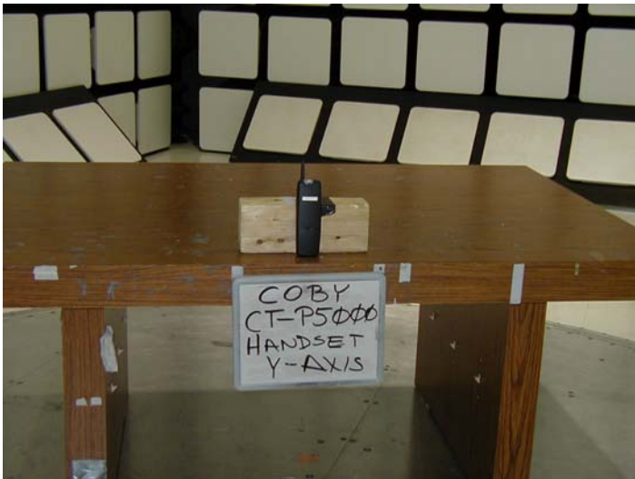
Radiated Emissions – Handset Y – Axis 10M Chamber
