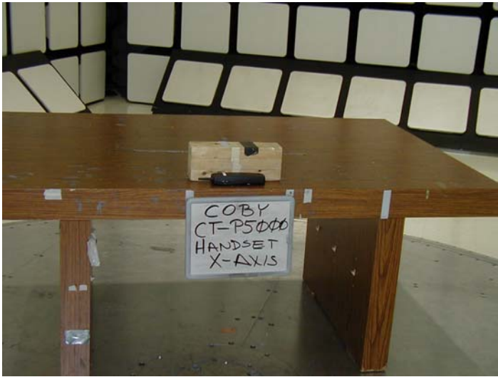
Radiated Emissions – Handset X – Axis 10M Chamber
