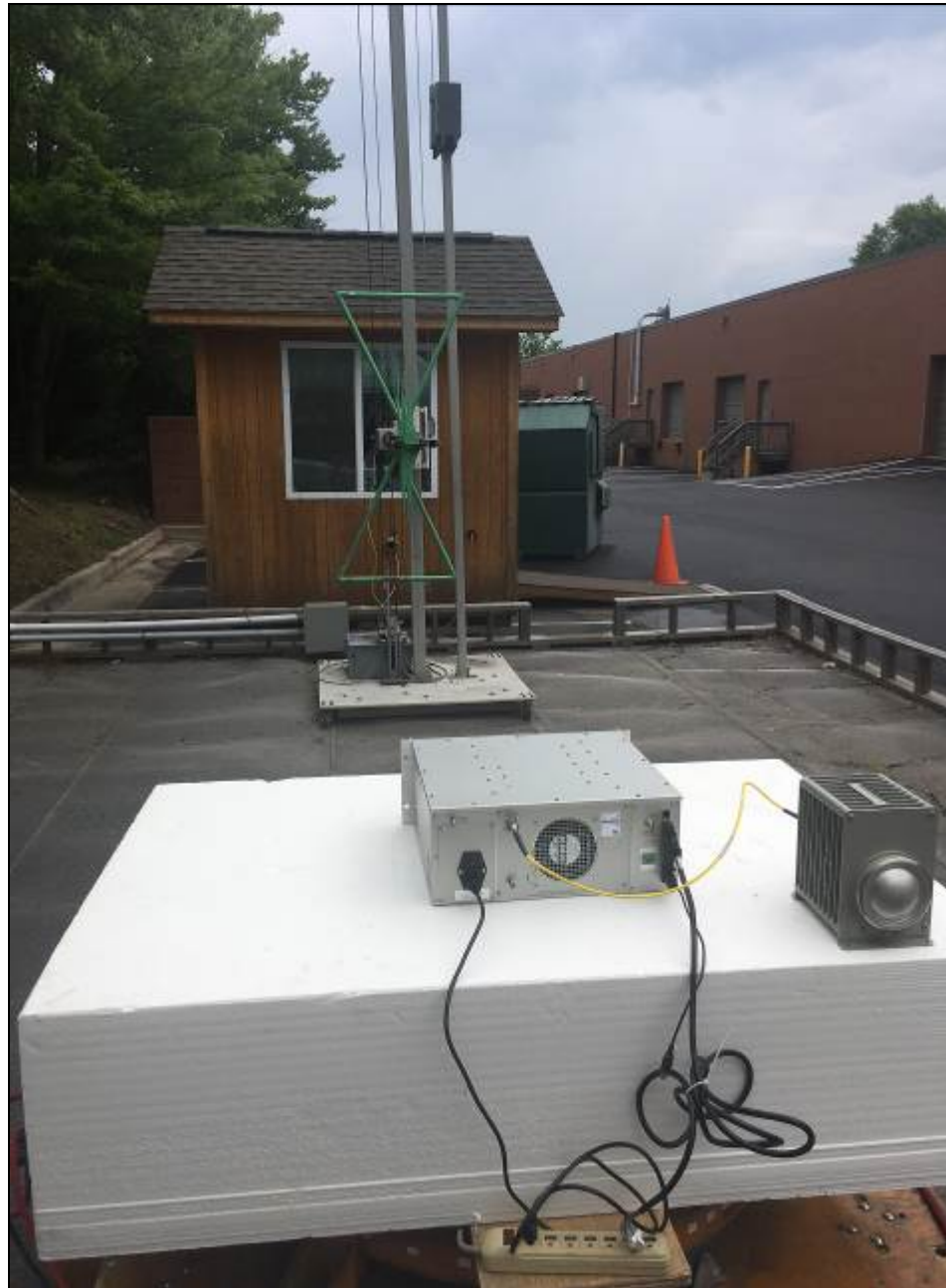
Photograph 4: Radiated Emissions (Spurious/Harmonics) – Back View (Below 1 GHz)
