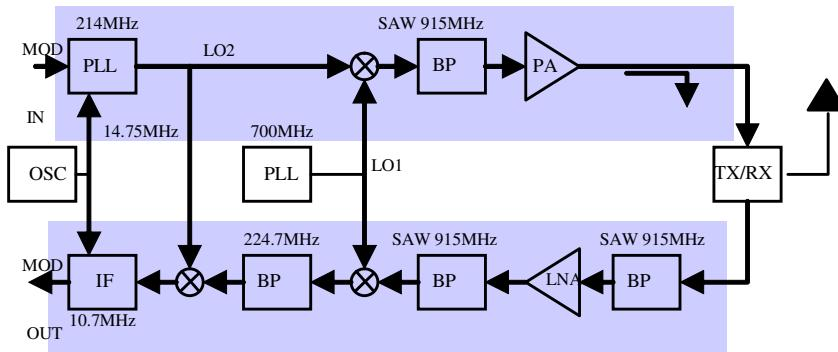
Figure 1: RFI-9256 RF Transceiver Block Diagram
