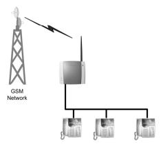
**Note:** When making the connections, the two-wire telephone cable polarity does not matter.
