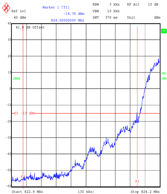
Title: Flextronic EUT: G32a FCC Part 22. Radiated Band Edge Comment A: 48122JD03 Operating in GSM 850, Bottom Channel, GPRS Mode. Date: 10.JUL.2006 12:31:39
