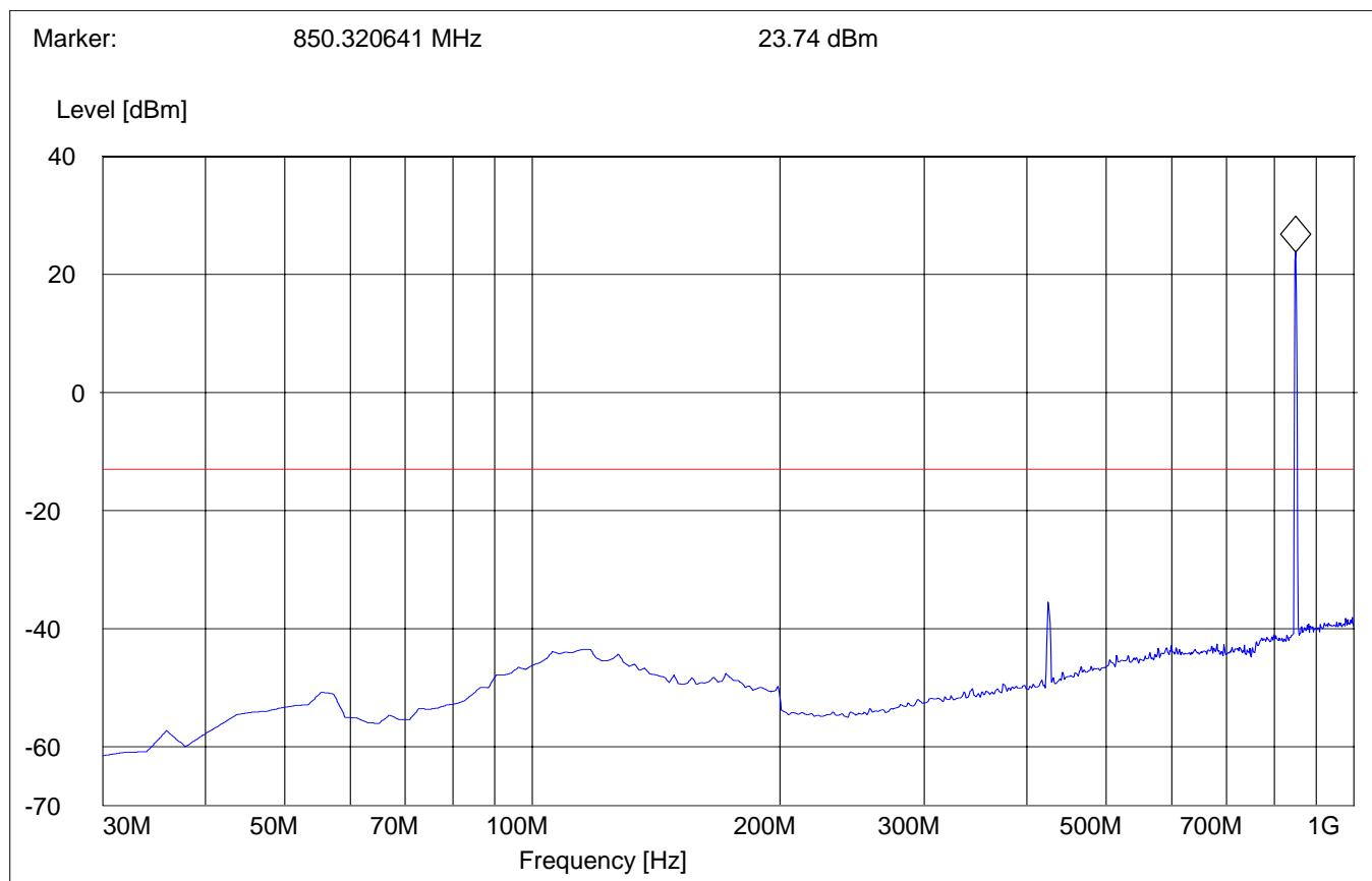
**RADIATED SPURIOUS EMISSIONS (GSM-850)****Tx @ 824.2MHz: 30MHz - 1GHz**
