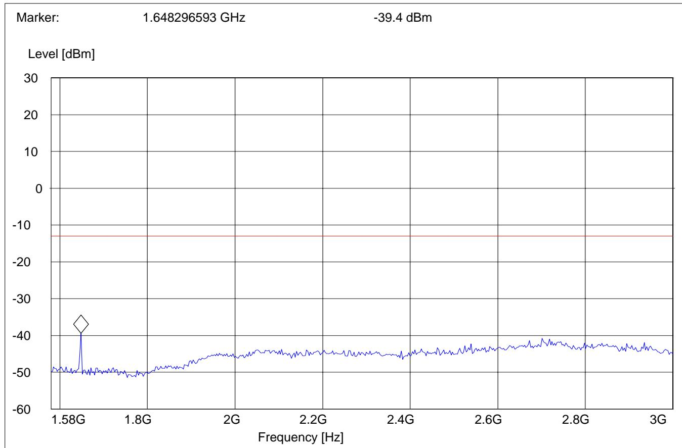
**RADIATED SPURIOUS EMISSIONS (GSM-850)****Tx @ 824.2MHz: 3GHz – 9GHz**
