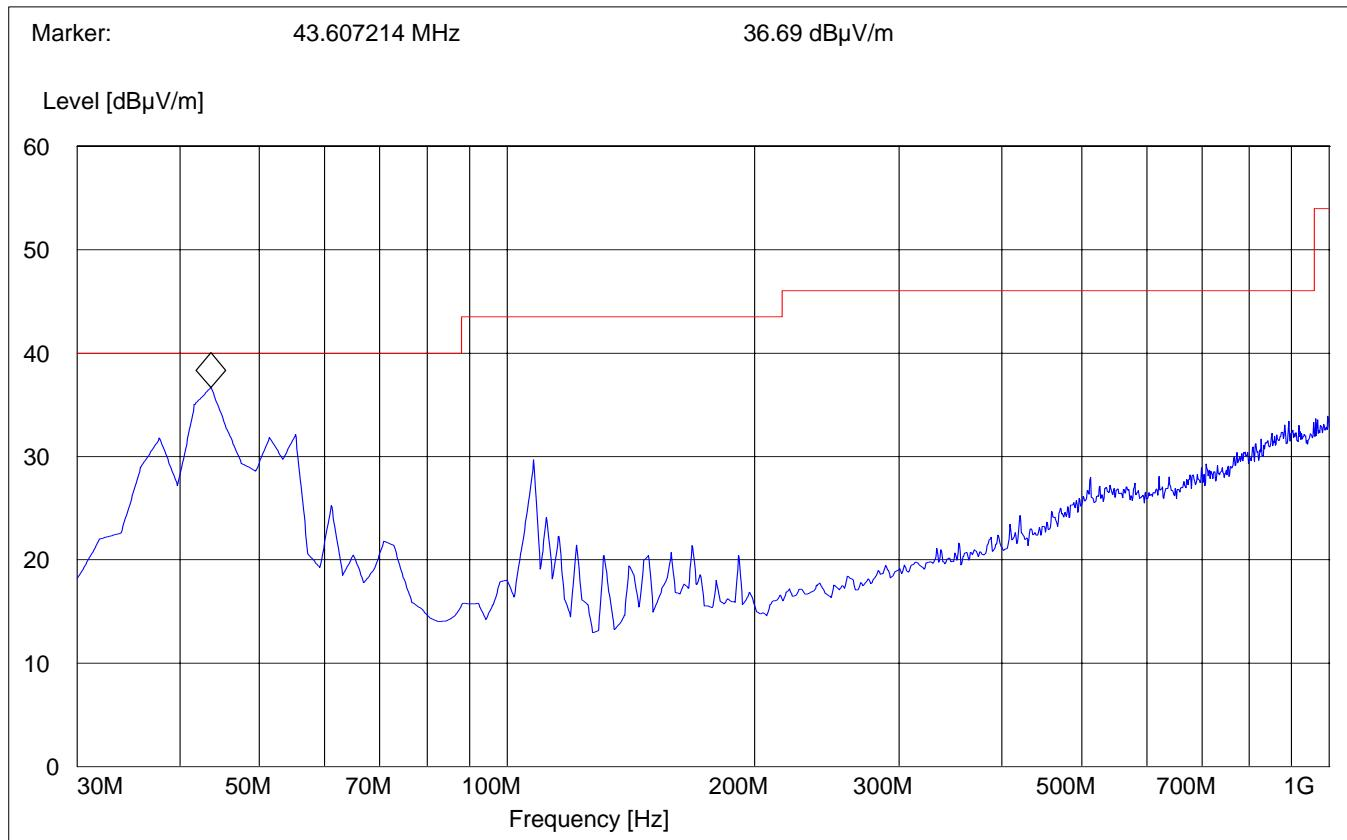
**RECEIVER RADIATED EMISSIONS****EUT in Idle Mode: 30MHz – 1GHz****Antenna: horizontal****SWEEP TABLE: "FCC 15 Spur 30M-1G"**
