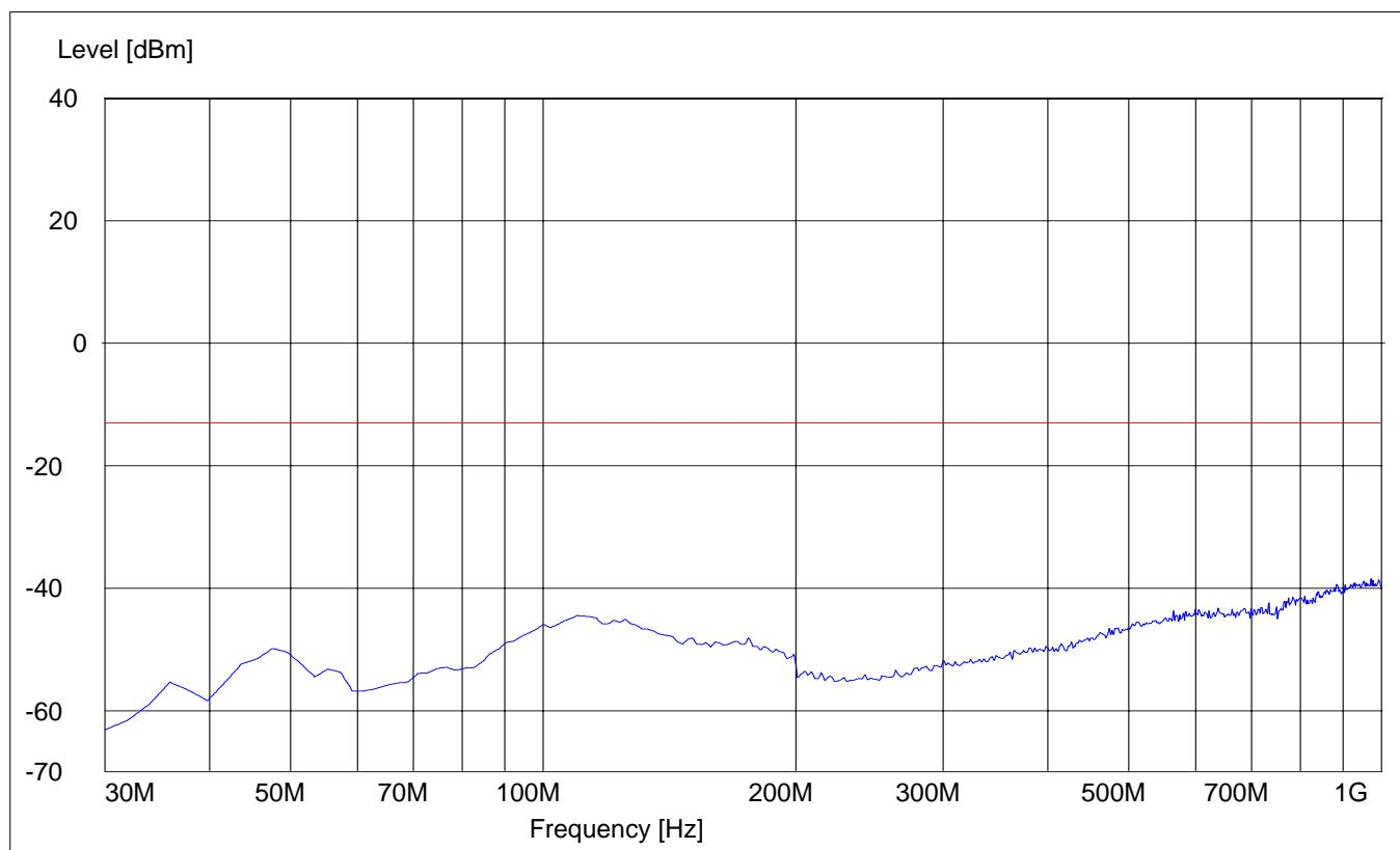
**RADIATED SPURIOUS EMISSIONS****Antenna: horizontal****Tx @ 1850.2MHz: 30MHz - 1GHz**
