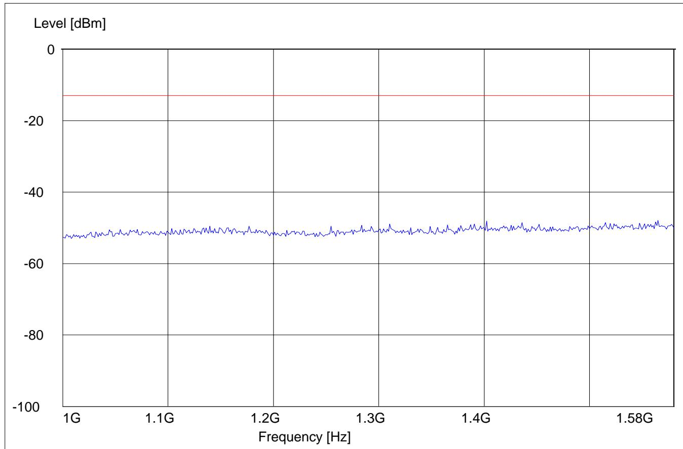
**RADIATED SPURIOUS EMISSIONS (GSM-850)****Tx @ 836.6MHz: 1.58GHz – 3GHz**
