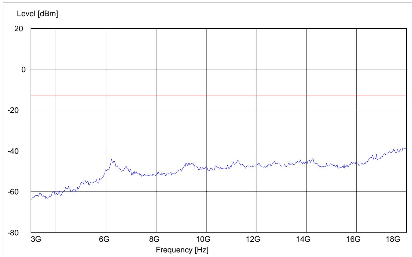
**RADIATED SPURIOUS EMISSIONS****EUT in Idle Mode: 18GHz – 19.1GHz**
