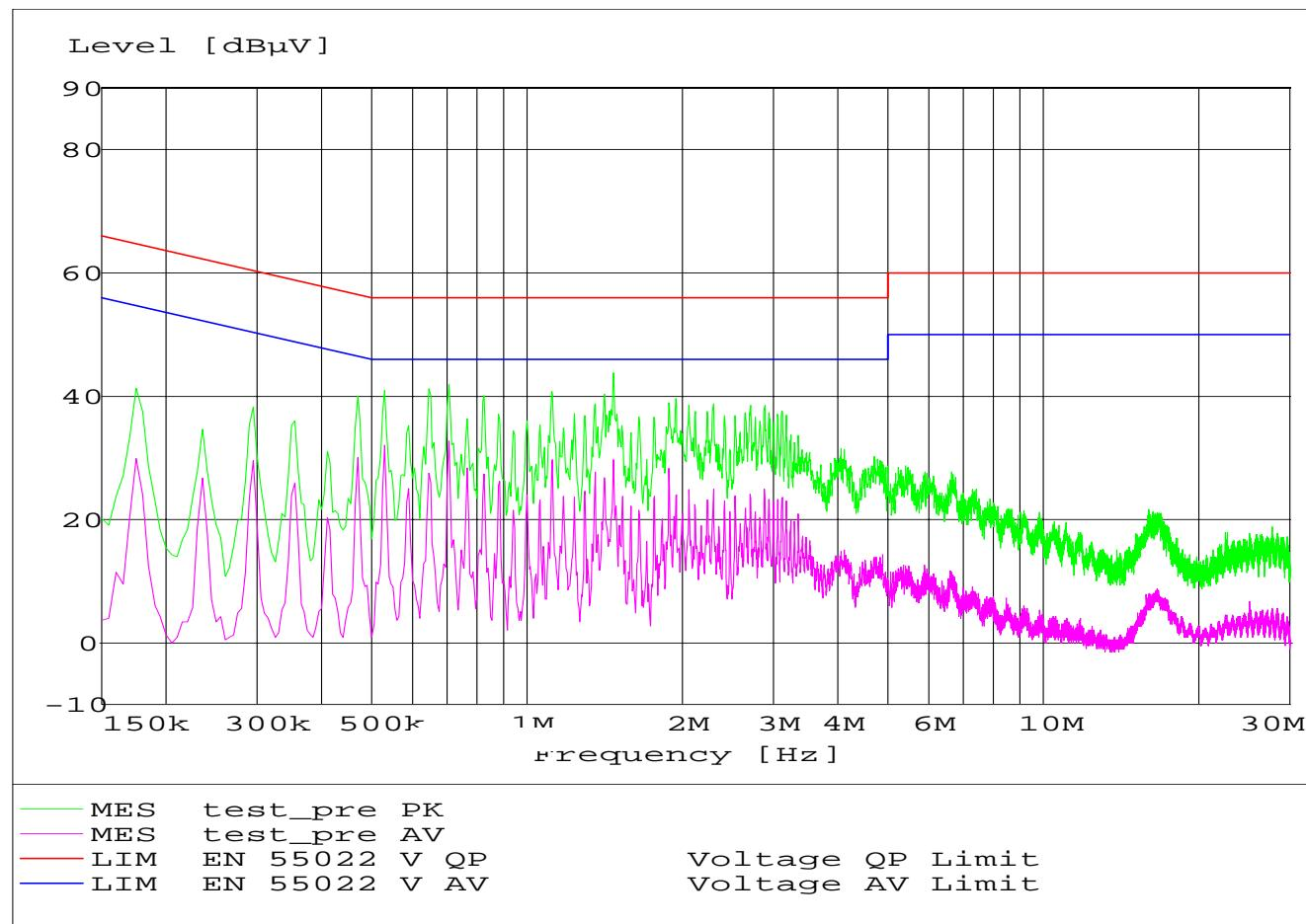
Measured with AC/DC power adapter
