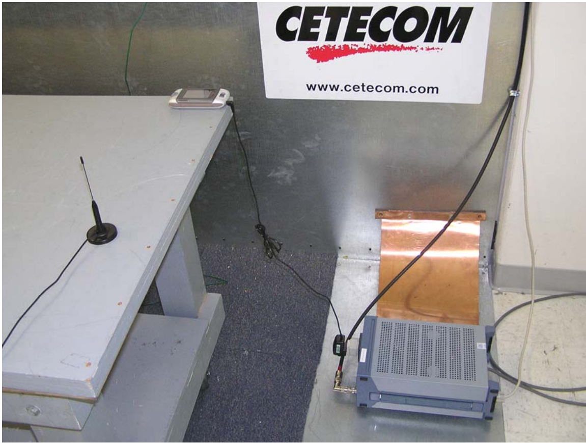
Test setup – AC Line Conducted Emissions
