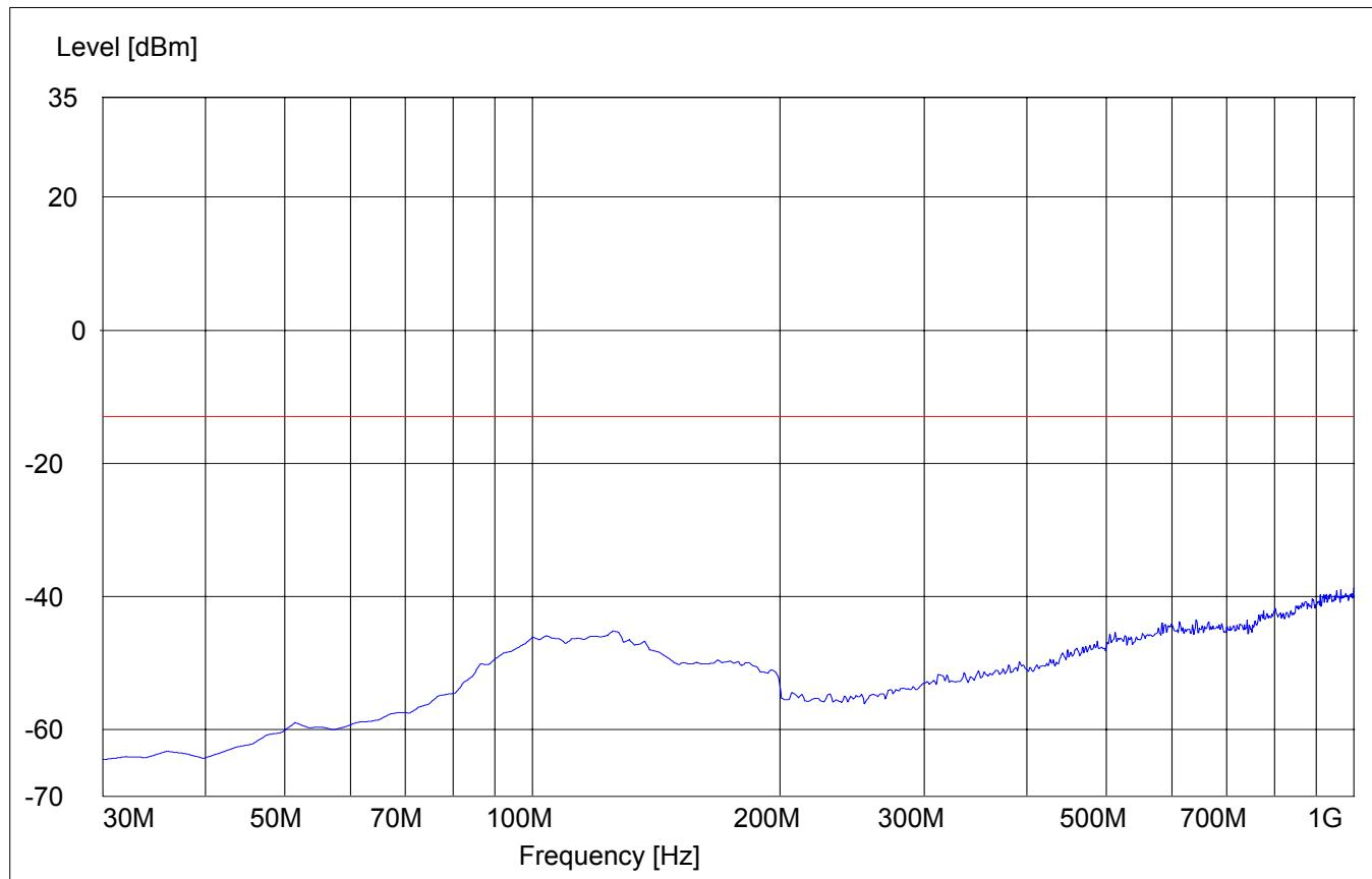
**RADIATED SPURIOUS EMISSIONS (IDLE MODE – GSM 1900)****Antenna: horizontal****EUT in Idle Mode: 30MHz – 1GHz**
