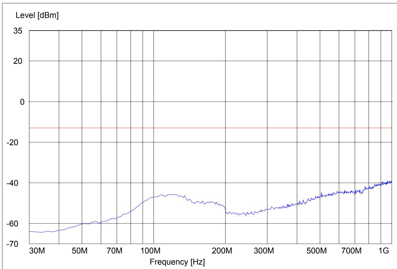
**RADIATED SPURIOUS EMISSIONS****Tx @ 1850.2MHz: 30MHz - 1GHz**
