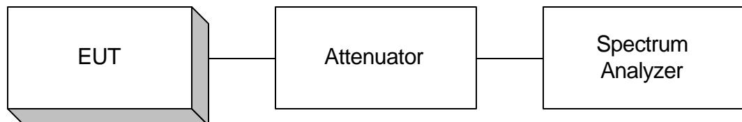
**Para. No. 2.1053 Spurious Emissions at Antenna Terminals**
