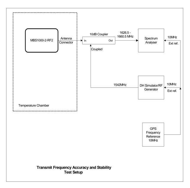
The transmitter frequency tracking to the DH frequency was tested using the DH test set over the MBS2-LP operating temperature. The transmitter was activated and its frequency was tuned over the operating band and measured to ensure that TX frequency deviation is within the spec limits. The test results are shown in the tables below. Note: all frequency offsets are normalized to  $20^{\circ}$ C
