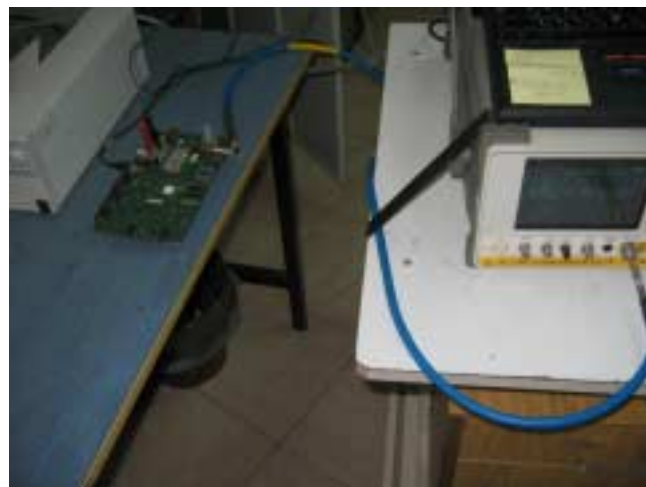
Photograph 7.2.2 Occupied bandwidth test setup
