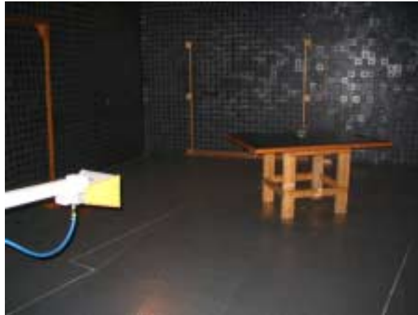
Photograph 9.2.2 Setup for radiated emission measurements, above 1 GHz
