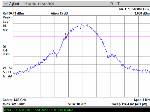
Plot 8.2.2 Occupied bandwidth test result at low frequency, lower reference point
