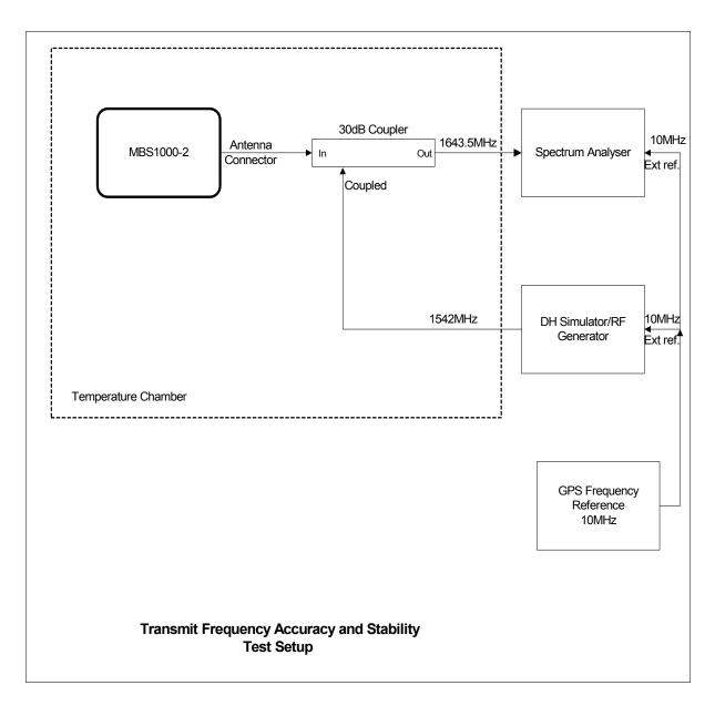
The transmitter frequency tracking to the DH frequency was tested using the DH test set over the MBS1000-2 operating temperature. The transmitter was activated and its frequency was tuned over the operating band and measured to ensure that TX frequency deviation is within the spec limits. The test results are shown in the tables below. Note: all frequency offsets are normalized to  $20^{\circ}$ C
