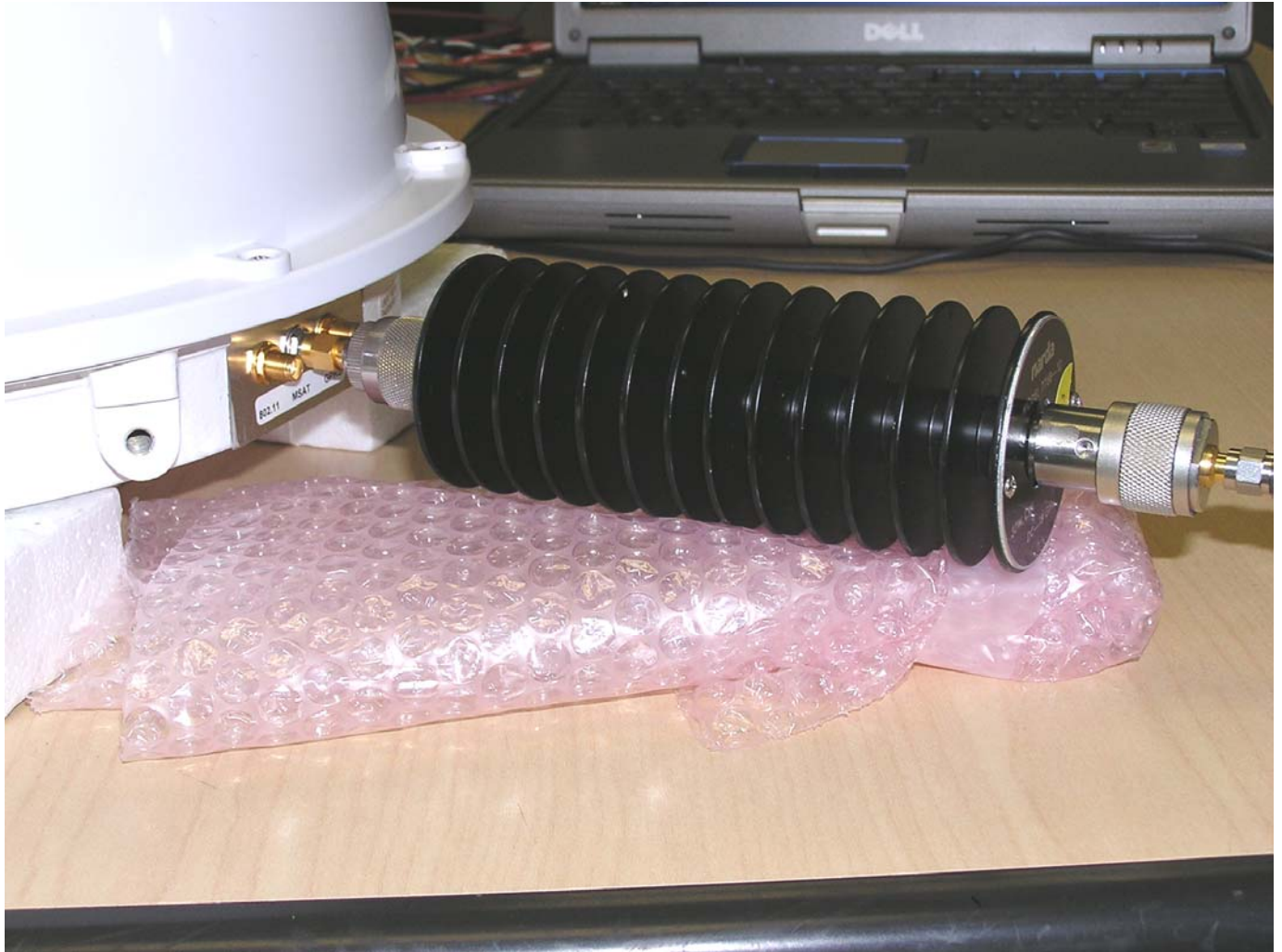
Test setup Conducted measurements (Temporary RF connectors provided for test purpose only)
