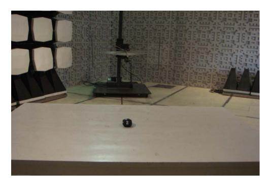
**Radiation Emission Test View For 1GHz-25GHz**
