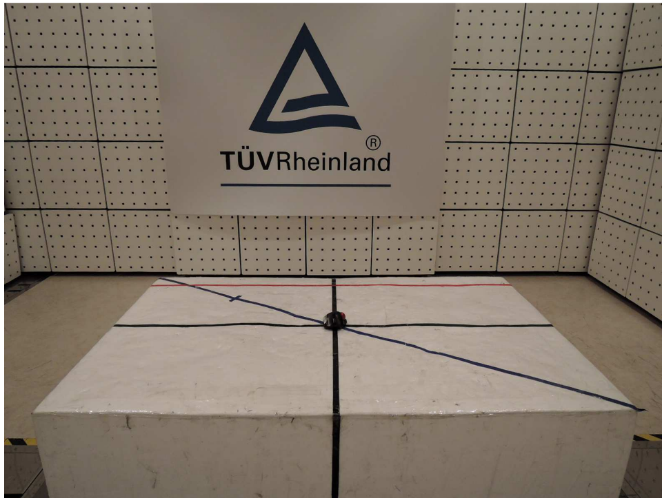
Photograph 1: Set-up for Spurious Emissions (Front View)
