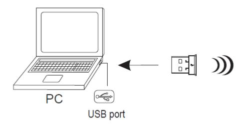
The 2.4Ghz RF mouse features a dual-way transmission technology which enables the mouse and the receiver auto-communication.
