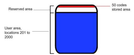
These codes allow TVTRX232-916 work as 50 different transmitters. Every transmitter can send up to 7 channels. These codes are fixed and not modifiable. In user memory area(201-2000) it's possible to store codes belonging to physical transmitters. To memorize a physical transmitter's channel can be use command 2 which allow to store a transmitter code via radio in a defined memory location.
