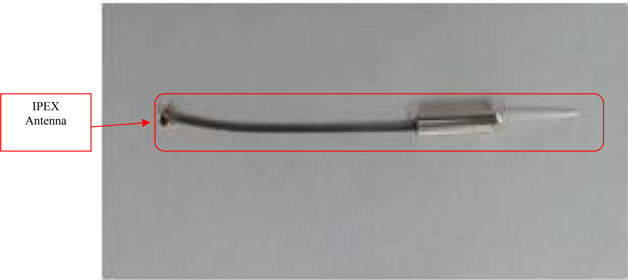
Note: the external antenna for EMW3161-E
