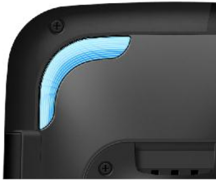
Figure 12 LED configuration of rear cover
