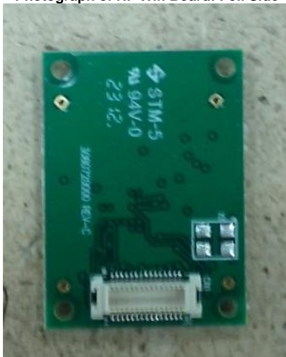
Photograph of RF Wifi Board: Foil Side
