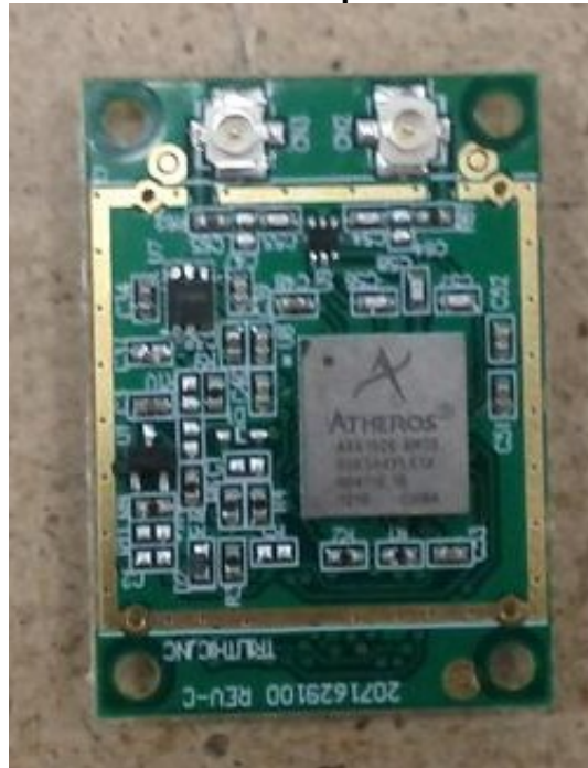
Photograph of RF Wifi Board: Component Side – Shield removed
