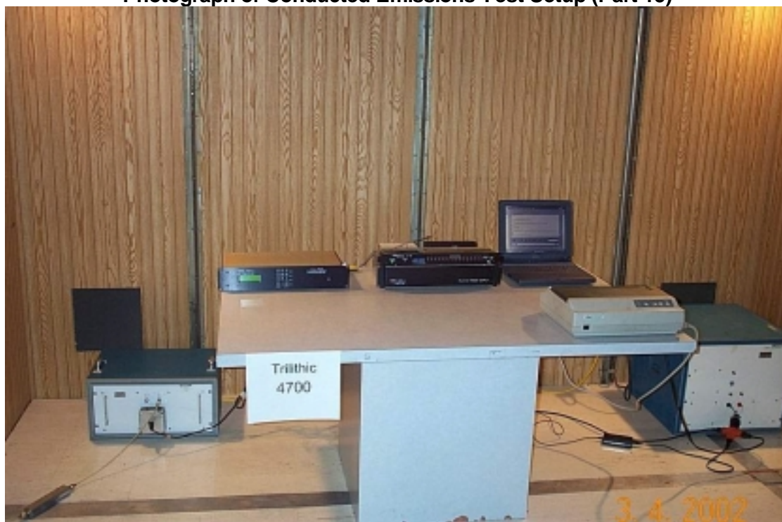
Photograph of Conducted Emissions Test Setup (Part 15)
