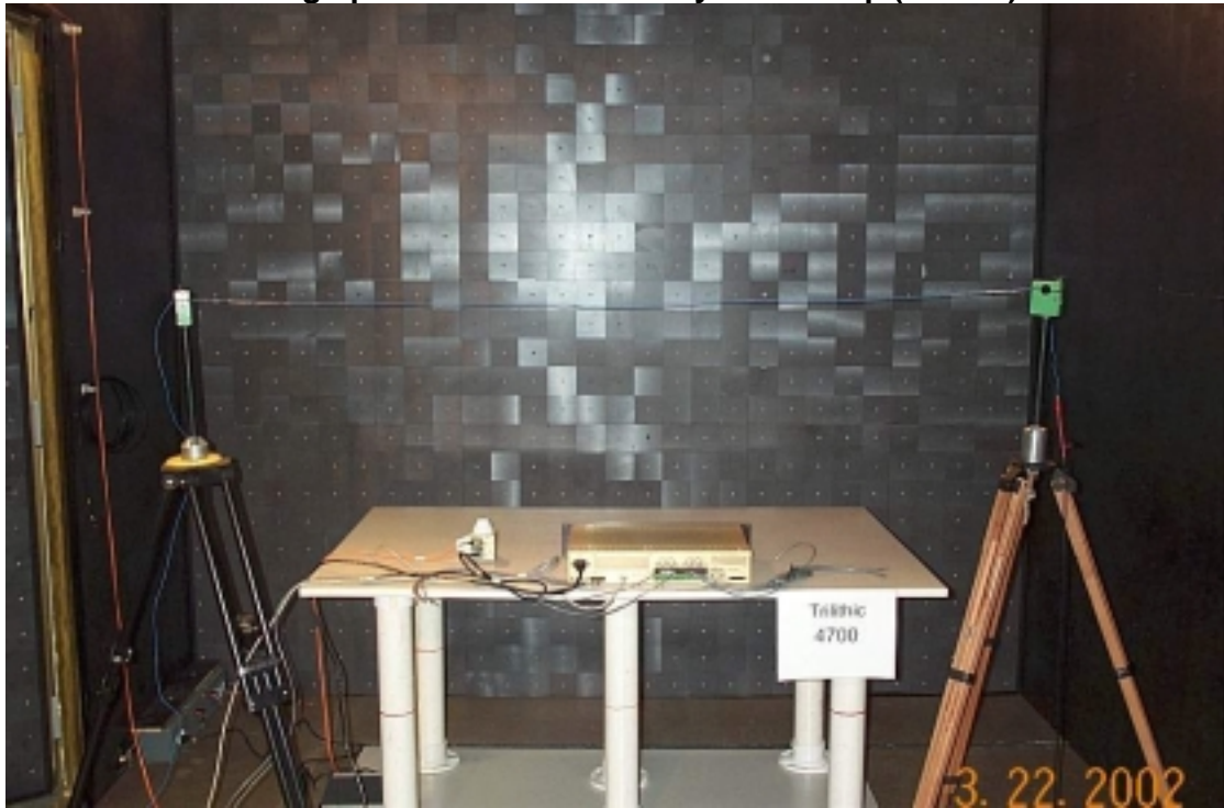
Photograph of Radiated Immunity Test Setup (Part 11)
