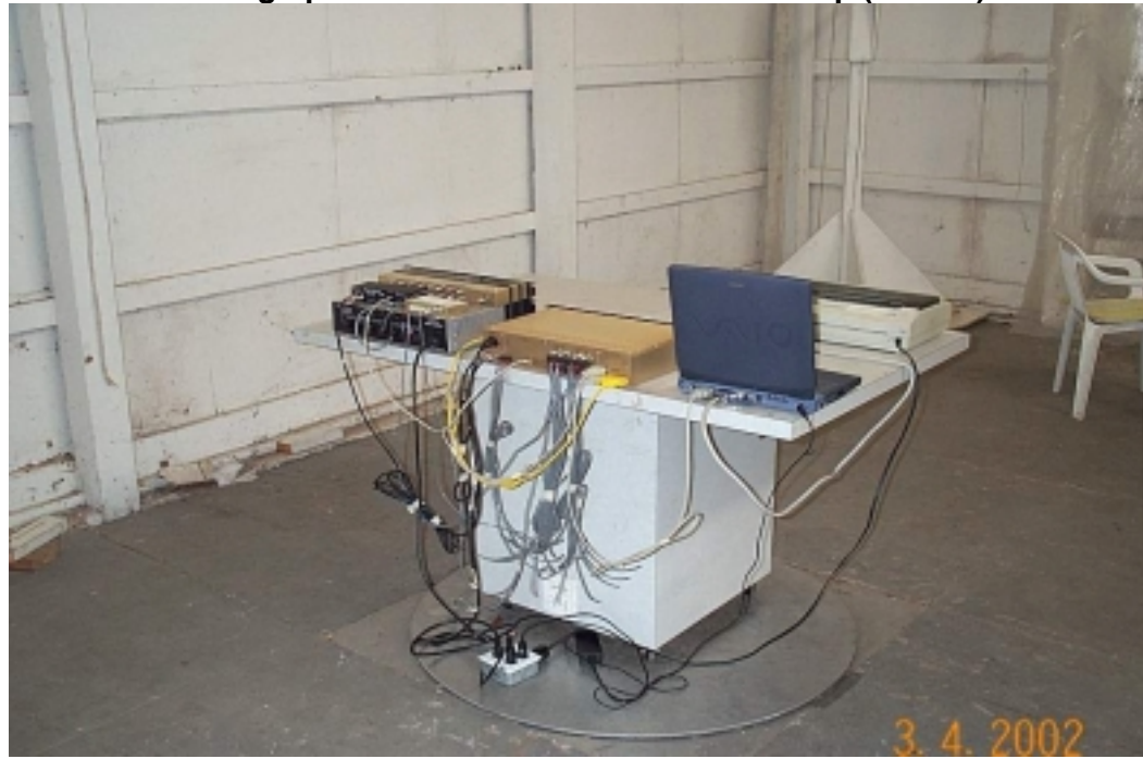
Photograph of Radiated Emissions Test Setup (Part 15)
