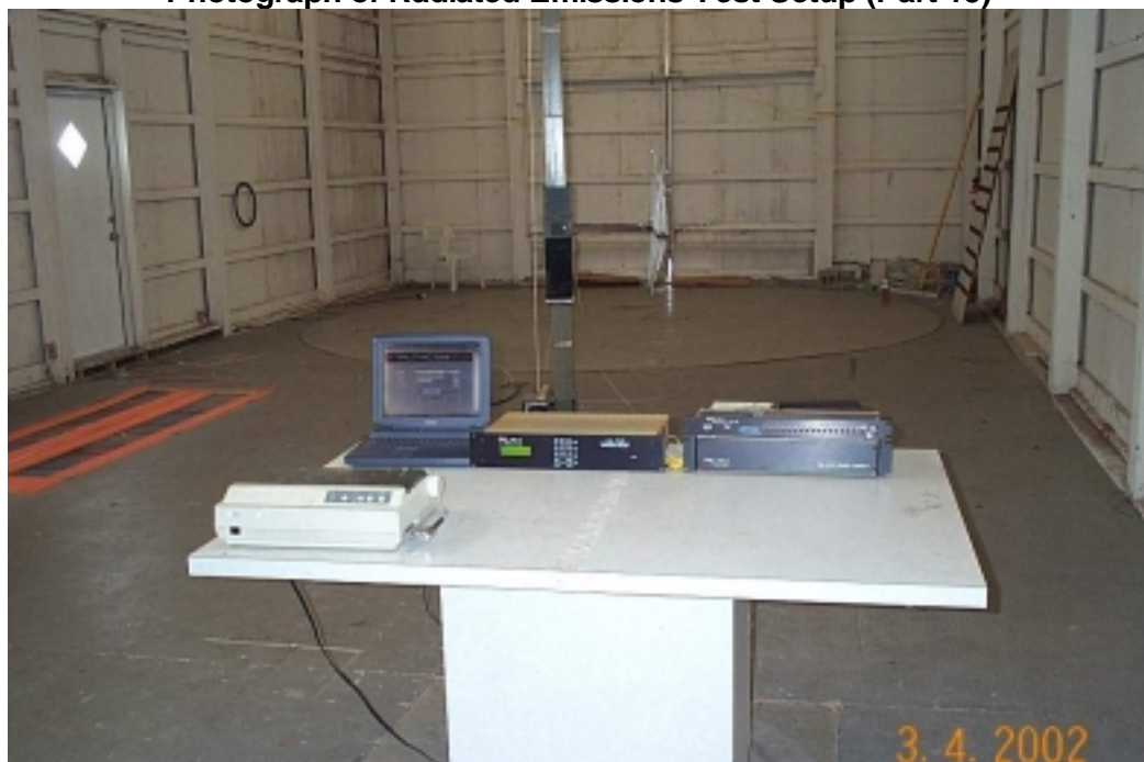
Photograph of Radiated Emissions Test Setup (Part 15)
