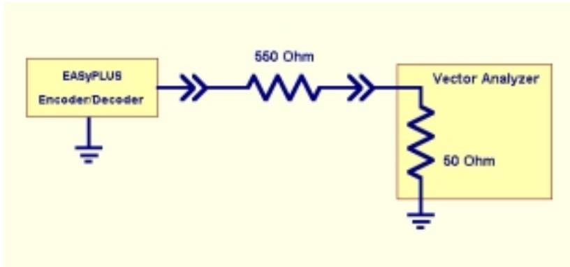
47cfr11.32-a-9-iii requires a +8 dBm signal into a 600 Ohm load, this is being measured on a 50 ohm Vector Analyzer, using a 550 Ohm series resistor for impedance matching. The voltage of 1.95 across the 600 Ohm load is proven to meet specifications by the following calculations/formulas.
