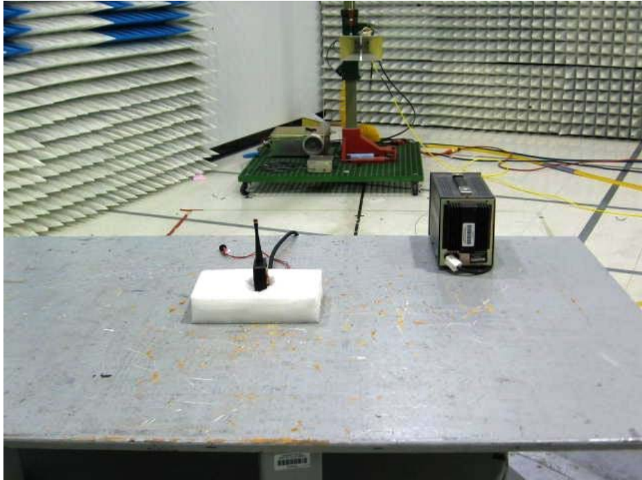
Radiated Emissions Test Configuration
