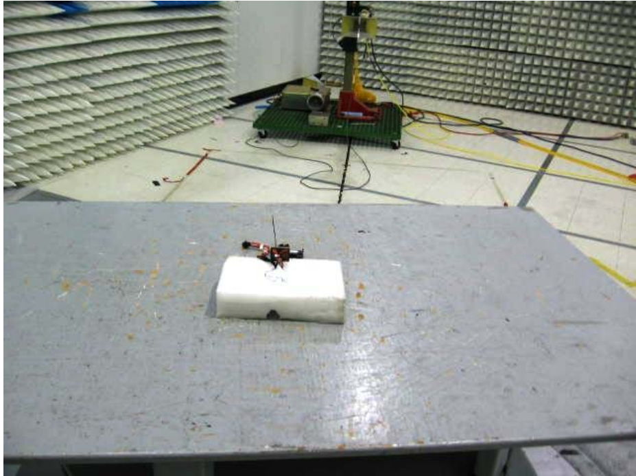
Radiated Emissions Test Configuration
