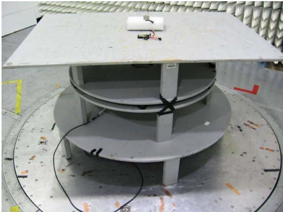
Radiated Emissions Test Configuration
