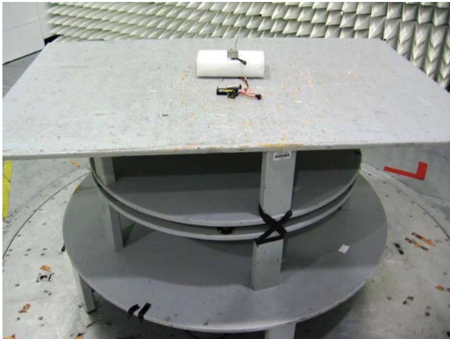
Radiated Emissions Test Configuration
