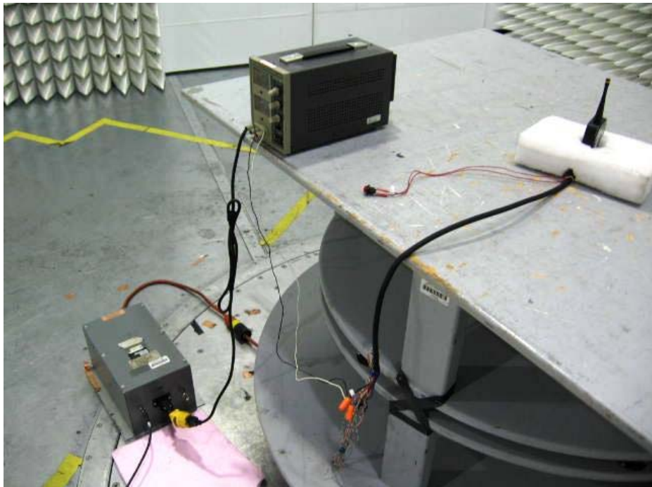
Conducted Emissions Test Configuration
