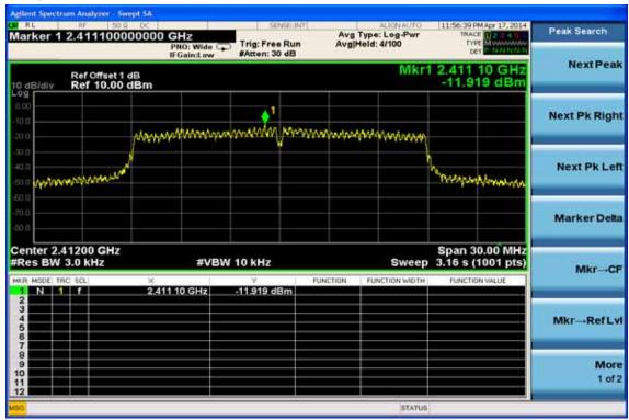
**Power Spectral Density Test Plot (CH-Mid)**
