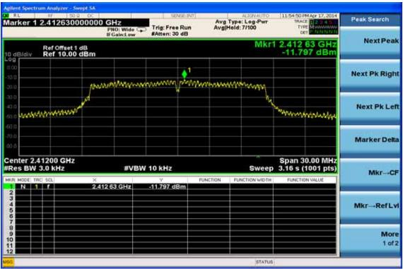
**Power Spectral Density Test Plot (CH-Mid)**
