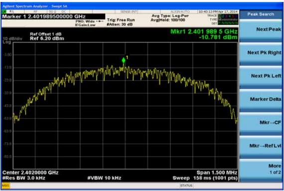
**Power Spectral Density Test Plot (CH-Mid)**
