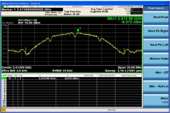
**Power Spectral Density Test Plot (CH-Mid)**
