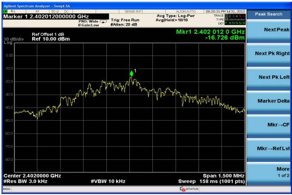
Power Spectral Density Test Plot (CH-Mid)
