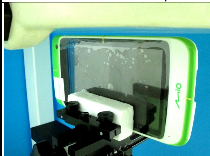
Right Side of EUT with 5 mm Gap
