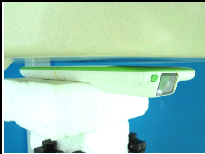
Front Face of EUT with 5 mm Gap
