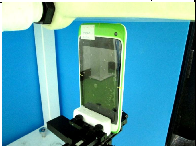
Top Side of EUT with 5 mm Gap
