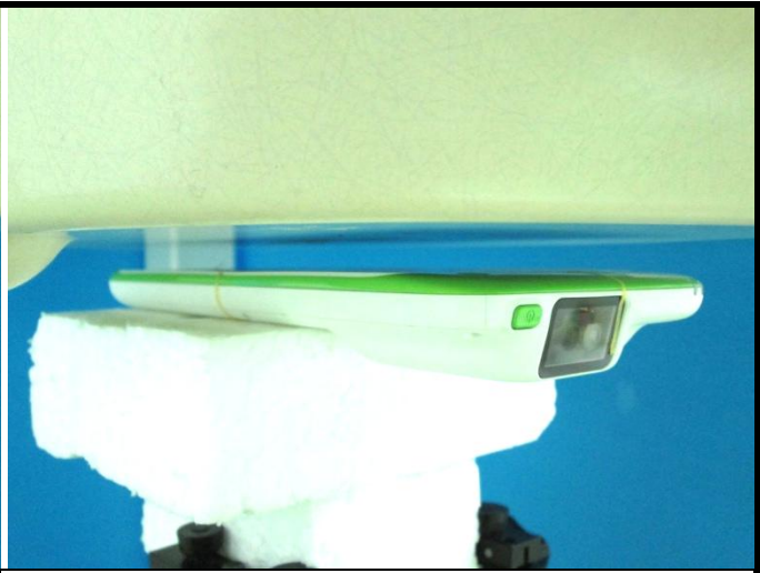
Front Face of EUT with 10 mm Gap
