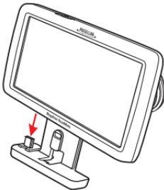
**Connect Power.** It is recommended that you connect the Magellan RoadMate using the vehicle power cable before using it for the first time. The internal battery will begin charging as soon as power is supplied to the Magellan RoadMate receiver through the vehicle power cable. (When the light on the vehicle power cable illuminates, it is properly connected to vehicle power. Note some vehicles require that the ignition be on before power is delivered to the power receptacle.)
