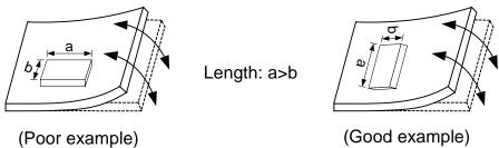
(b) Products (A,B,C,D) shall be located carefully so that products are not subjected to the mechanical stress due to warping the board. Because they may be subjected to the mechanical stress in order of A>C>B≒D.
