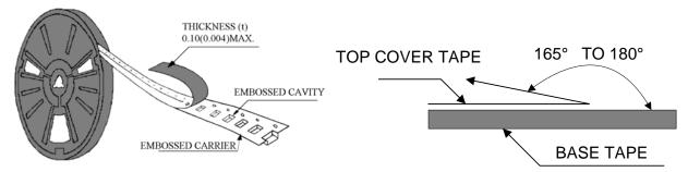
The force for peeling off cover tape is 10 grams in the arrow direction.
