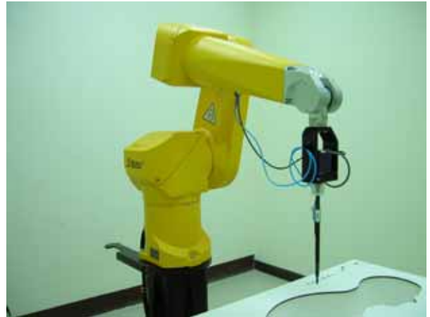
Fig. 5.2 Probe setup on robot
