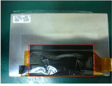
2. Add a AL-foil L85\*W49.2\*0.085T on the LCD, cover the LCD FPC P/N: 343164700100
