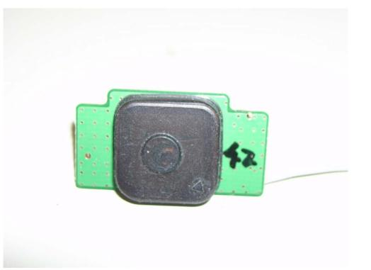
7.Expose this 2 place at LED board, and add 2 conductive cloth,15mmX20mm, connect LED board to LCD shielding
