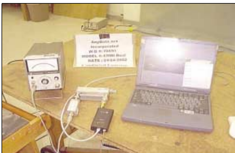
Carrier Output Power Test Setup
